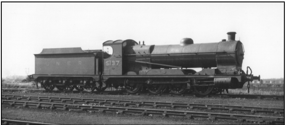
LNER class Q4 0-8-0 no. 5137. Built by Kitson & Co. in 1904 as GCR class 8A. Superheated with 21in cylinders and piston valves in 1921. The original 3,250 gallon tender was replaced with the 4,000 gallon tender in 1924. Height reduced to LNER loading gauge in 1930 (as shown in photo). Shed allocation in 1948 was Barnsley. Withdrawn 1949 as no. 63214.
