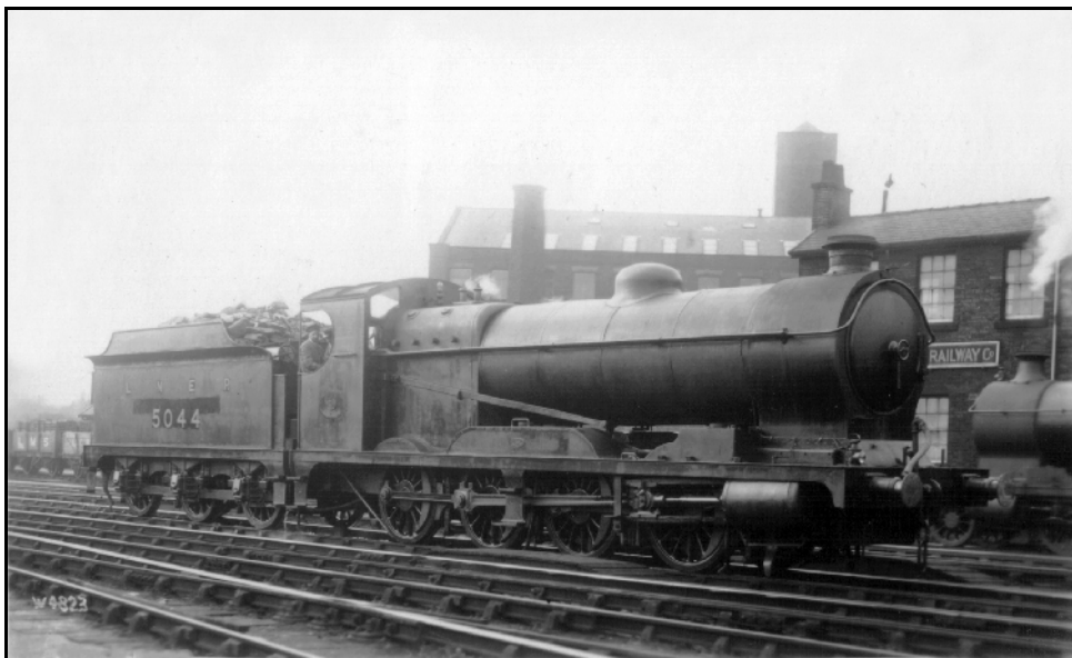
LNER class Q4 0-8-0 no. 5044 at Guide Bridge in 1924. Built by the GCR at Gorton in 1909 as class 8A with 4,000 gallon tender. Superheated 1924. No anti-vacuum valve. Low dome and short 1' 3" LNER chimney fitted (as shown in photo). Rebuilt as Q1/2 (longer bunker) in 1944. Withdrawn 1958 as 69931 at Selby shed. photo: Whitworth 4823
