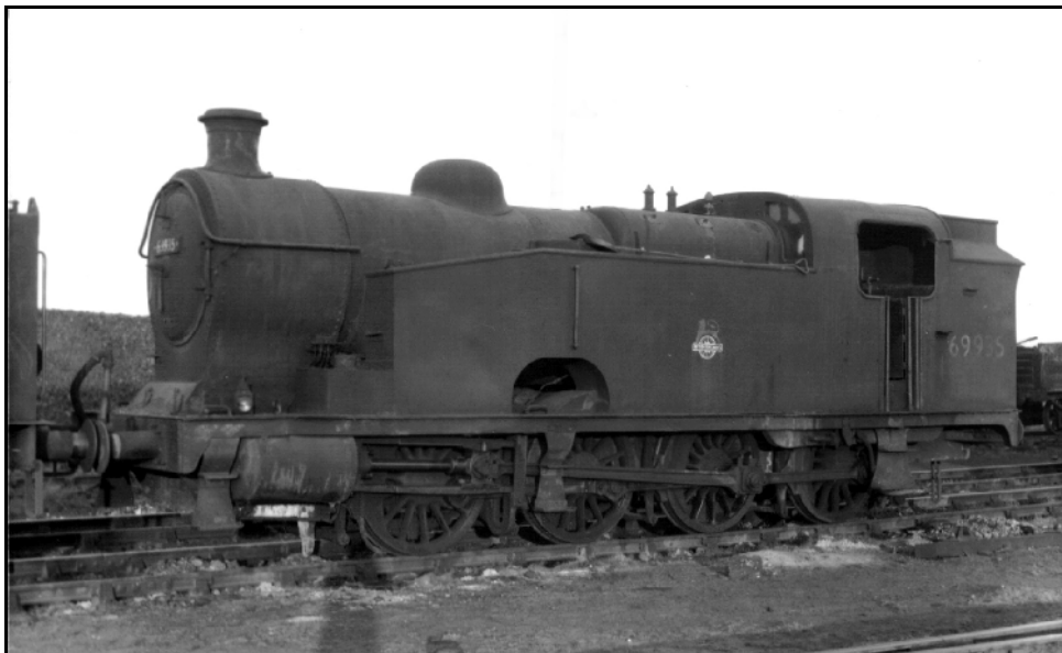
BR class Q1/2 0-8-0T no. 69935. Built by Kitson & Co. in 1904 as GC class 8A no.147. Became LNER class Q4 no.5147. Rebuilt as Q1/2 (longer bunker) in 1945. This was one of the Mexborough locos and one of the last to be withdrawn in 1959 from Frodingham shed. photo: E. Lowden Collection
