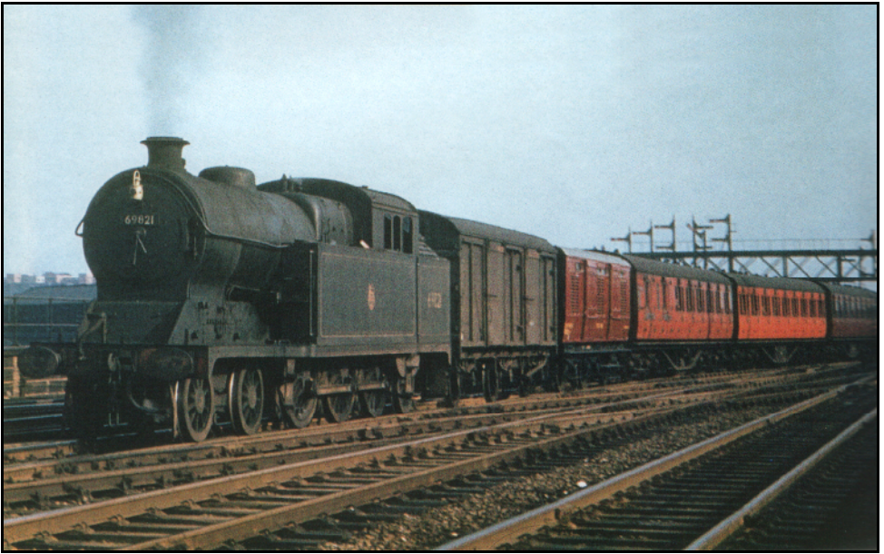
Above – BR class A5/1 4-6-2T no. 69821 at Derby in May 1959. Built by the LNER at Gorton in 1923, from a GCR order, as no. 5006. photo: J.B. McCann
