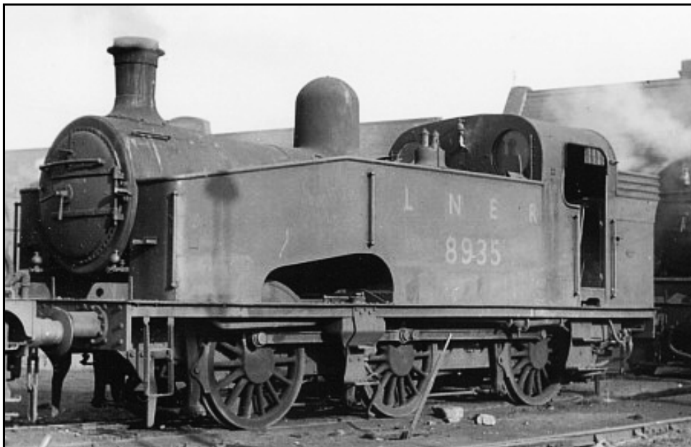
Gresley's LNER class J50/2 0-6-0T no.8935 at Annesley shed in 1948. These small locos had a T.E. of 23,635 lbs, almost the same as a class A5 4-6-2T. photo: M.Peirson
