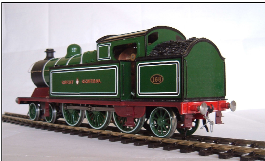
A gauge 1 model of GCR class 9N 4-6-2T no.168 made by Christopher Ardron to a Paul Forsyth design. See additional notes on opposite page. photos: Christopher Ardron
