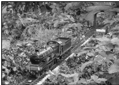
GCR class 13 4-2-2 no.967. Model by Arthur Parsey. Electric motor via stud contact.
