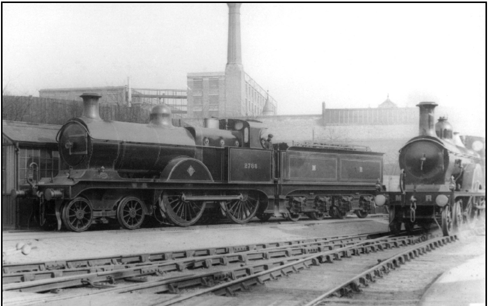
Johnson obviously considered his customary flowing curves and a Belpaire boiler to be mutually exclusive, nevertheless his class 3 'Belpaire' was a very handsome locomotive. Note the subtly raised running plate and matching tender. photo: Photomatic
