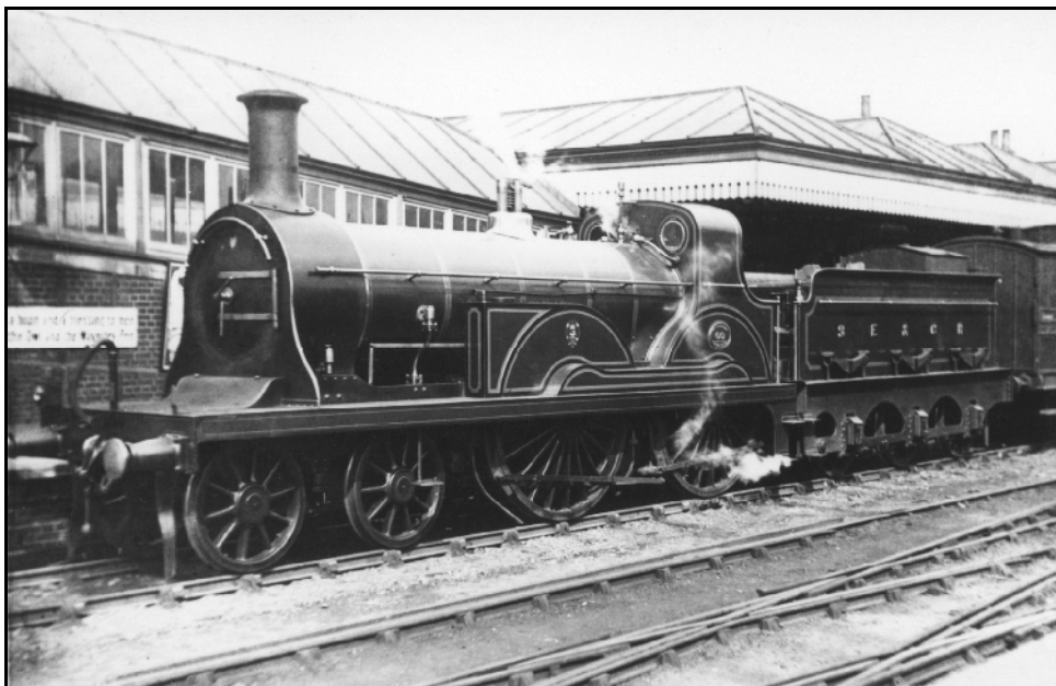
Straight-back domeless boilers and rounded 'wrap-over' cabs typified the "Stirling look". James Stirling's F class 7' express passenger 4-4-0 no. 60 for the South Eastern Railway, complemented by all the finery of the Wainwright SE&C livery - but still with the SER crest on her splashers.
