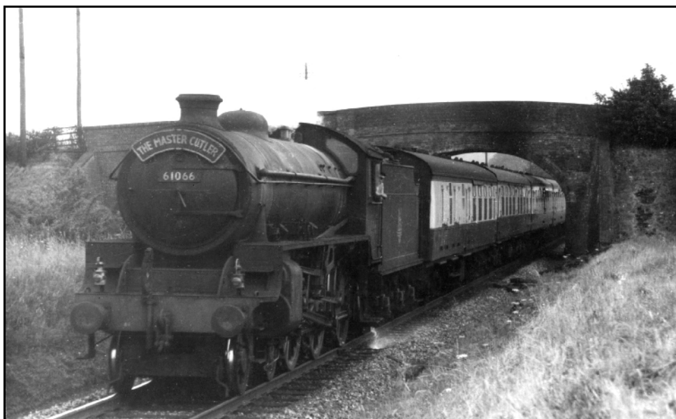
BR class B1 4-6-0 no. 61066 passing under Lee Road bridge on the approach to Saunderton with the up 'The Master Cutler'. The brick double bridge (the down line bridge is hidden by the locomotive) has since been replaced by a single span modern structure. photo: unknown
