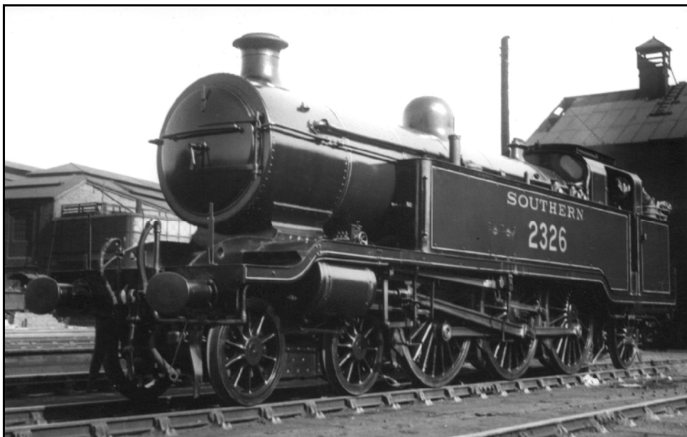
Class J2 no.326 'Bessborough' (built 1912) was the second of two 4-6-2Ts built by the LB&SCR at Brighton. It is seen here as SR class J2 no.2326. The original D.E.Marsh design, as used for class J1 no.325 'Abergavenny' (built 1910), had been modified by his successor, Robert Billinton.
