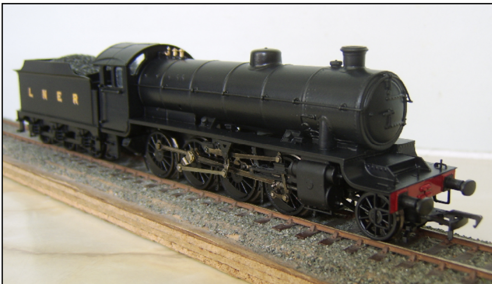
Graeme King's model of a class O1 2-8-0 made by modifying the Bachmann class O4 model.
