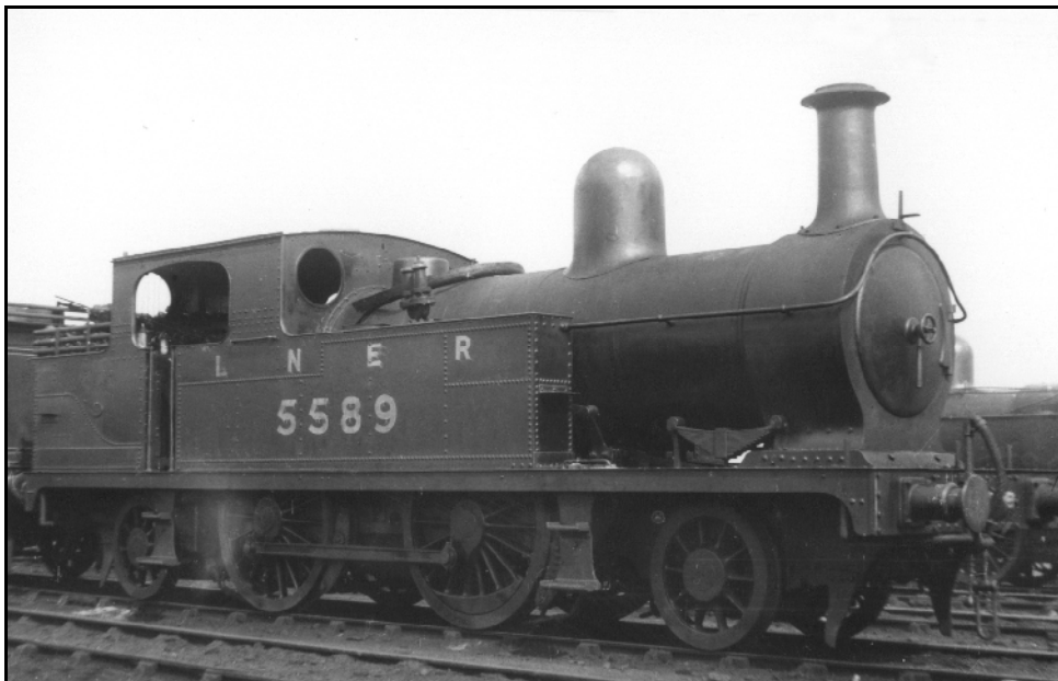
In LNER days class F1 2-4-2T no. 5589 is still in unrebuilt form. It was the last of the class to receive its Belpaire boiler in 1929. photo: Photomatic
