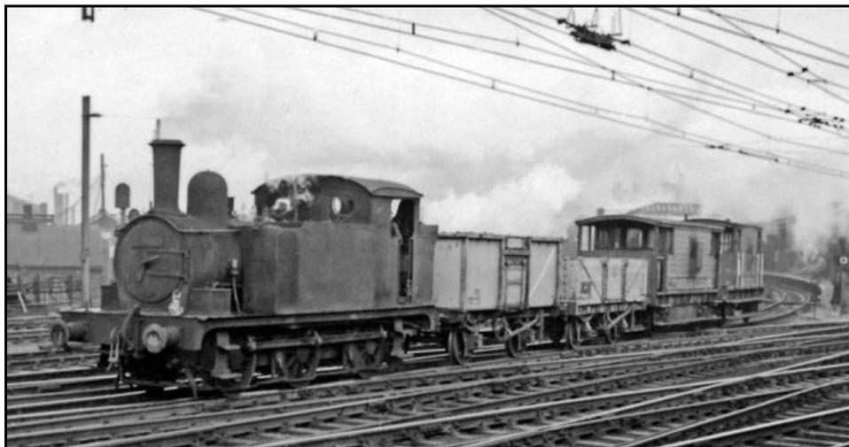
*Ex-GER Holden class J69 0-6-0T no.68571 with a short pick-up goods near Stratford on 23 Dec 1959. With a change of location this could be the Buckley branch pick-up! photo: © Ben Brooksbank*
