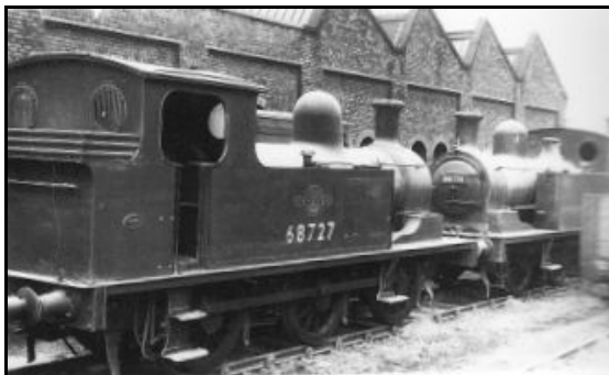
Ex-NER J72 0-6-0 tanks nos.68727 and 68714 at Bidston shed in Sept. 1959. Both have reduced height chimneys for working the Buckley branch. photo: H.C.Casserley
