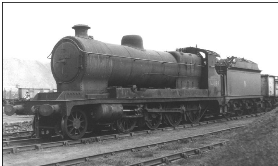
above: BR class O4/3 2-8-0 no.63783 at Pontefract in May 1958. Built by the North British Loco Co. in May 1918 for the ROD as no.1880, it entered LNER ownership in Feb.1928 as O4/3 no.6589 (distinguished from O4/1 by not having a vacuum brake pipe on the buffer beam). It became no.3783 in 1946 and no.63783 in 1948. It remained unrebuilt and was withdrawn in Dec.1962. Note the bent frame at the front end, a common feature of the O4s.
