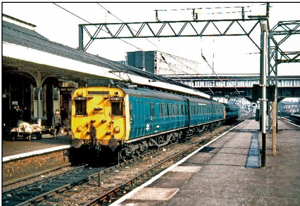
*Manchester-Altrincham 1,500 volts DC suburban units M28581M-M29657M-M29238M and M29239M-M29669M-M28590M at Altrincham station on 10<sup>th</sup> April 1971. The changeover to 25kV AC took place just a few weeks later on 3<sup>rd</sup> May.*
