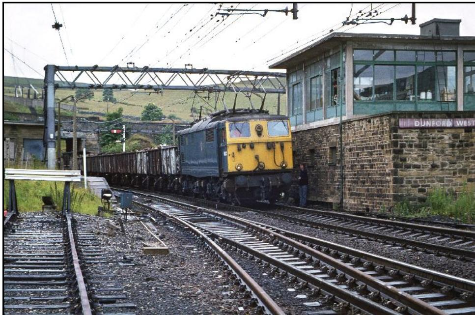
*A signal failure at around 13:00 on the last day meant that trains had to stop at the Dunford West signal box for instructions. Here a single Bo+Bo stands alongside the box with an up train of scrap bound for Tinsley yard. Note the semaphore signals visible beyond the 5<sup>th</sup> wagon that are standing guard at the end of the up yard.* photo: Adrian Freeman
