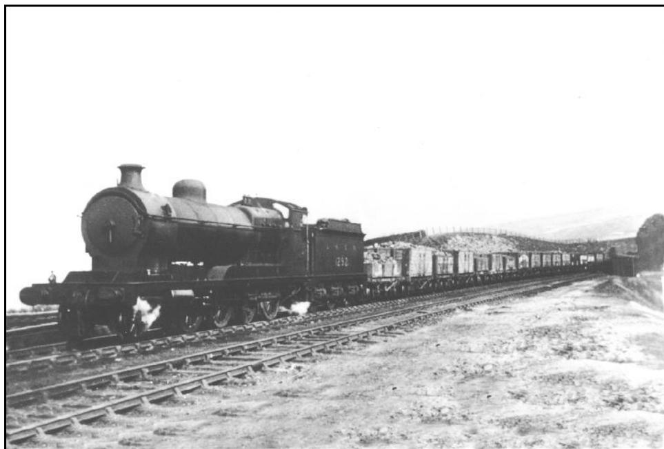
*LNER class O4/3 2-8-0 no.1292c approaching Penistone with a down coal train made up of an assortment of wagons in 1924. This ex-ROD loco was built by the North British Loco Co. in June 1919 and entered service on the LNER in Jan.1924 being renumbered 6292 in Aug.1924. Rebuilt as O4/8 in May 1944 and withdrawn in Nov.1963 as no.63853. It is a pity that the photo isn't clear enough to identify the wagons. The first wagon is a 4-plank GC vehicle. Would this be used for carrying coal?*
