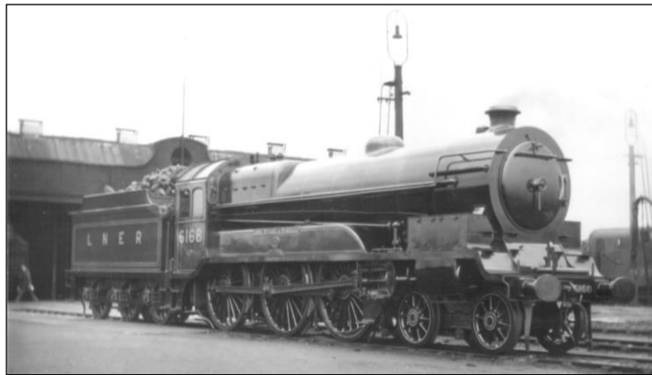
LNER class B3/2 4-6-0 no.6168 Lord Stuart of Wortley at Neasden. Rebuilt with Caprotti valve gear.
